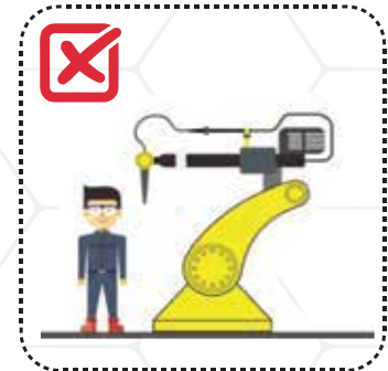
No Guarding to Protect Employee
