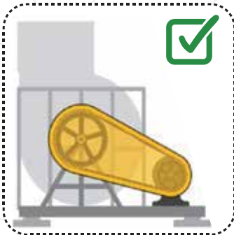
Install Guarding at Rotating Part
