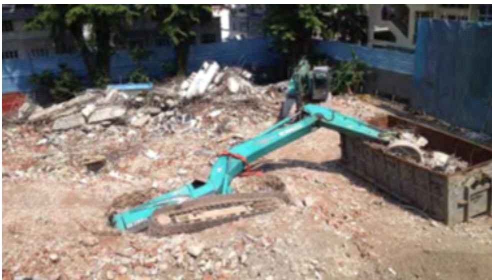
Rajah 5.1 Jentera yang tenggelam di kawasan tanah tidak padat ( Ground Conditions for Construction Plant Strategic Forum for Construction, Good Practice Guide, London, 2014 )
