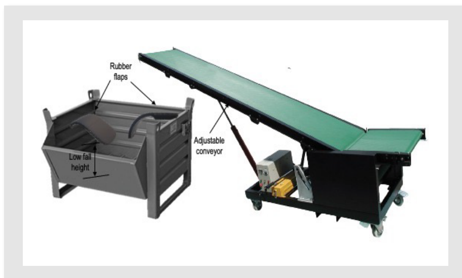
Figure 6.10: Reducing drop height and using rubber flaps to slow down fall speed and absorb impact.
