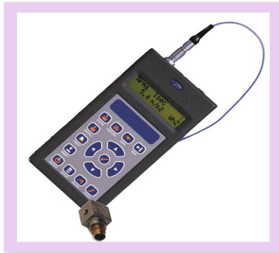
Figure 6.22: Example of vibration meter.
