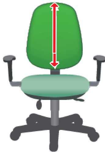
Figure 7.10 Backrest height should be sufficient to accommodate and support the backrest of the user thus allowing postural change and promote active sitting
