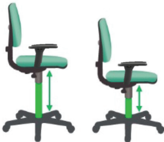
Figure 7.6 Adjustable height chair relies on the pneumatic gas lift cylinder (indicated with bright green colour)
