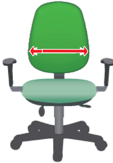
Figure 7.11 Sufficient backrest width provides support to the upper body of the user, allowing users to rest during recline sitting
