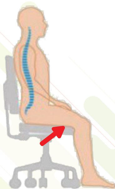
Figure 4.7 Contact stress caused by compression between of hard surface (seat pan) on soft tissues (back of thighs)
