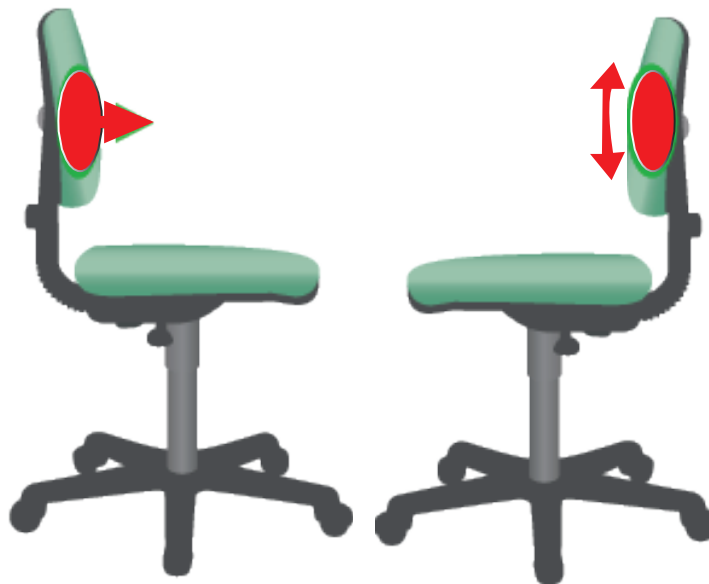
Figure 7.13 Adjustability of lumbar support may include depth adjustment (left) and height adjustment (right)
