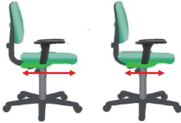
Figure 7.7 Adjustable seat pan of the chair allow user to slide-adjust outward (front) or inward (back) depending on the buttock–popliteal length of the user
