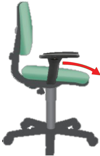
Figure 7.9 Seat pan angle adjustability provides the user the flexibility to carry out active movement-sitting, varying between forward or backward tilt posture
